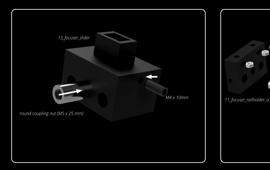
Insert the round coupling nut M5 x 25mm (mine had a diameter of 7.9mm) into the center hole of the focus slider (13\_focuser\_slider). It should be a tight fit and you may have to resort to some brute force.
