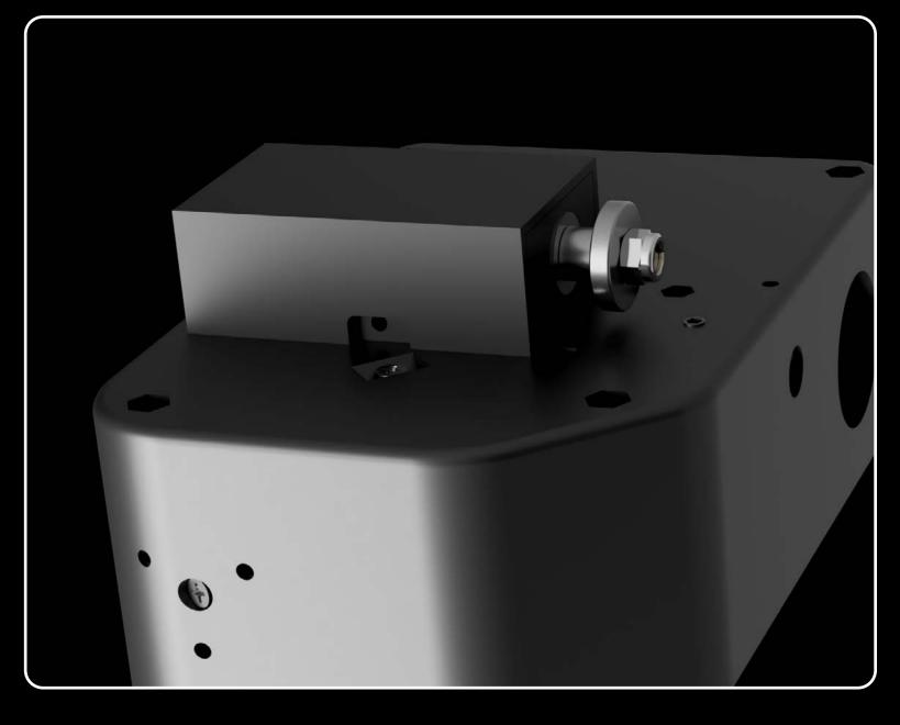
Place a M5 washer over the cylinder screw and screw on the Knurled nut. Make sure not to screw it to tight against the washer. The washer should be able to move a little bit.
