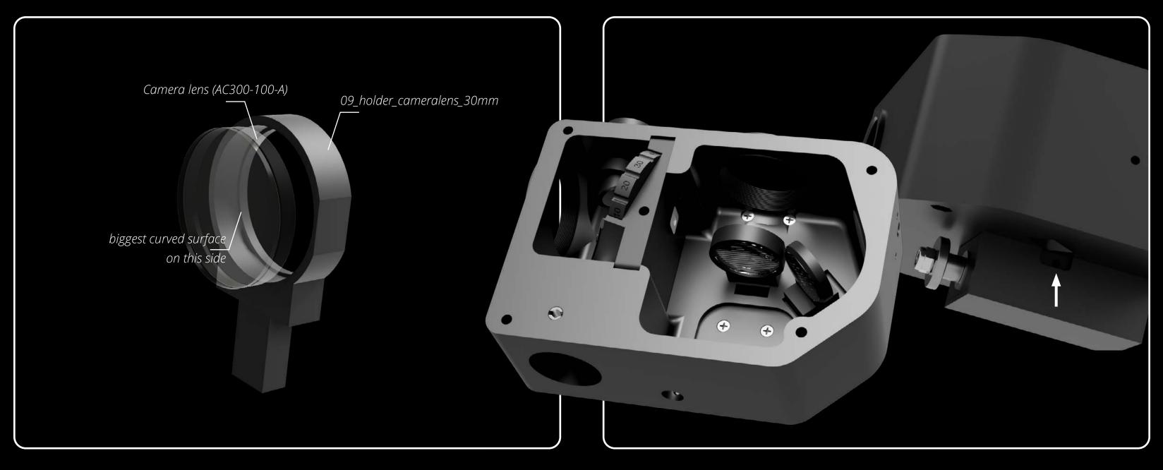
Push the 30mm camera lens (AC300-100-A) into it's holder. Note the orientation of the lens and holder.
