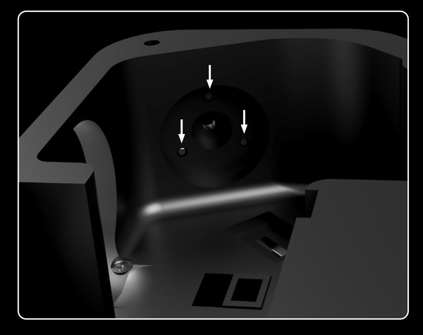
Press the mirror into the main mirror holder. Wear gloves so you will not damage the mirror! If you feel the mirror is not secure in it's holder, then use a small droplet of glue on the backend.
