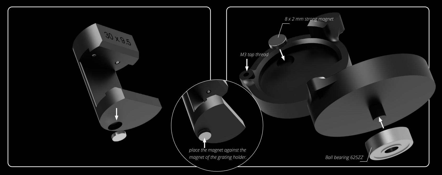
Put a small amount of glue (epoxy) in the hole at the bottom of the grating holder. Insert the small permanent magnet (diameter 8 mm, thickness 2 mm) in the hole. Make sure it does not stick out. The bottom of the holder needs to be flat.
