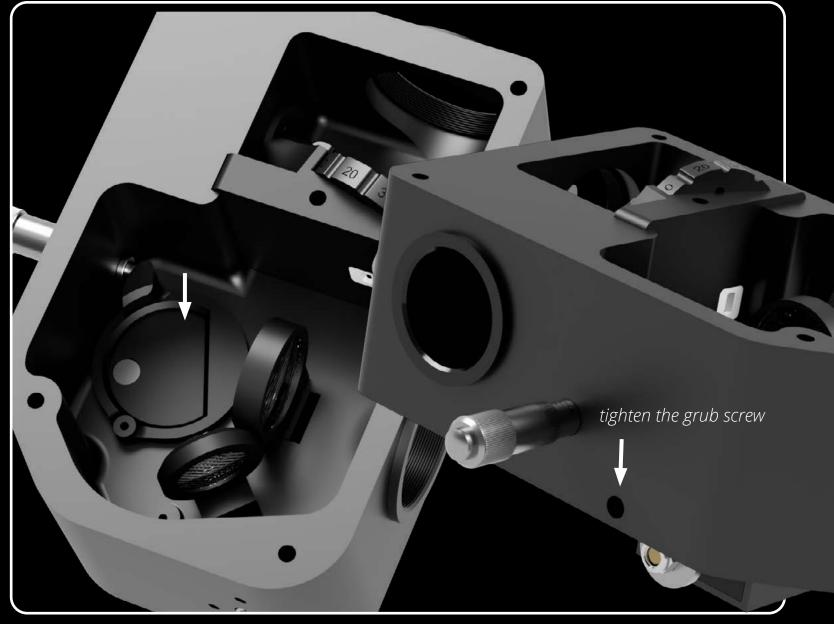
Test that there is a good fit between the grating holder and the turn table. Make sure that the two magnets place the grating holder correctly into the turn table.
